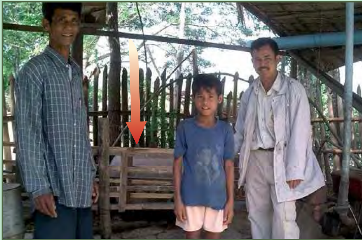
Guard covering a moving belt of a rice mill machine
