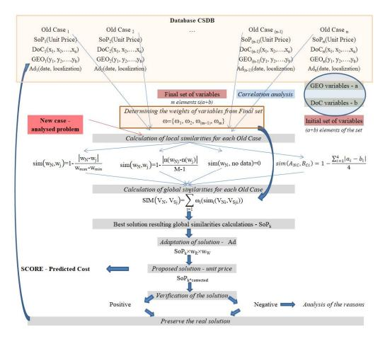
Figure 1. Algorithm used in the method proposed.
