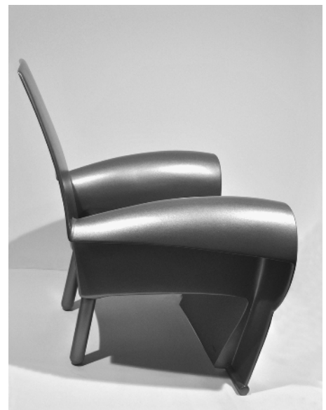
Figure 1.15 Richard III, designed by Philippe Starck (1982–1984), manufactured by Baleri Italia as a single shell molded structure in rigid polyurethane and finished with polyurethane enamel in metallic silver. 36¼ inches wide; 32¼ inches deep; 36 inches high (92 cm wide; 82 cm deep; 91.5 cm high). Photography by Jim Postell, 2011.
