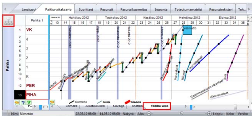
Fig 34 Construction Phase Schedule /22/
